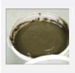
BentoPaste is an expanding and crack bridging isolation mastic formulized by mainly natural sodium bentonite, rubber compound and special polymer additives. It is a one component formulation requiring no need of mixture of additional water. BentoPaste is easy to apply either with the help of putty knife, trowel or by hand. It adheres to surface even in vertical applications and provides continuous impermeable waterproofing layer on the applied surfaces.
